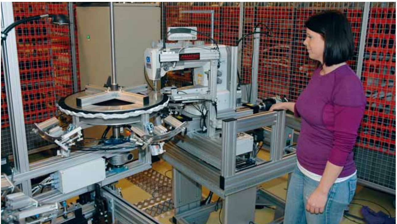
Ekornes invests both to increase its level of manufacturing automation and enhance the skills of its staff. Here is the world's first sewing robot, which recently went into operation at the Stressless® factory. The new robot sews covers to the base of the Stressless® Jazz and Stressless® Blue models. Michelle Sandvold is the machine's operator.
