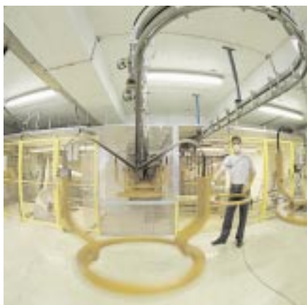
Lakking av Stressless® understell/ Vanishing and staining of Stressless® bases
